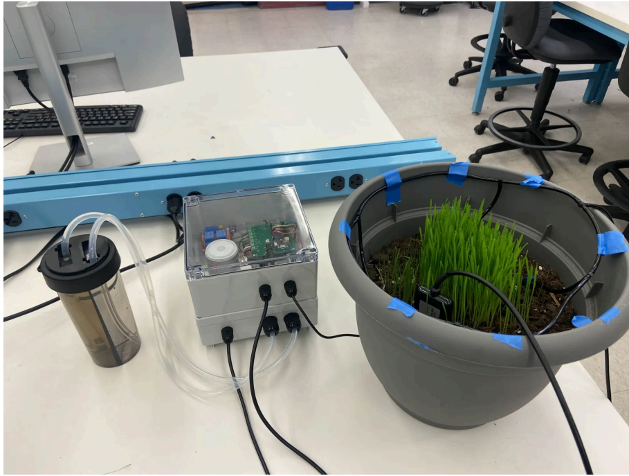
Figure 19: This image shows a viable setup with the Nuture hardware system. The fertilizer/water reservoir is shown on the left, the hardware enclosure in the center, and the pot with the watering system and NPK system on the right.
